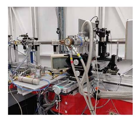
The high vacuum cryogenic vapour deposition system for in-situ simultaneous Raman and X-ray diffraction at the Brockhouse sector (BXDS). Credit: John Tse
