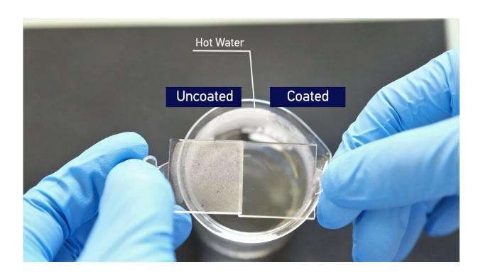
When exposed to steam from hot water, fogging is observed on the uncoated plastic substrate (left), while no water vapour condensation is seen on the coated sample (right). Credit: Nanyang Technological University
