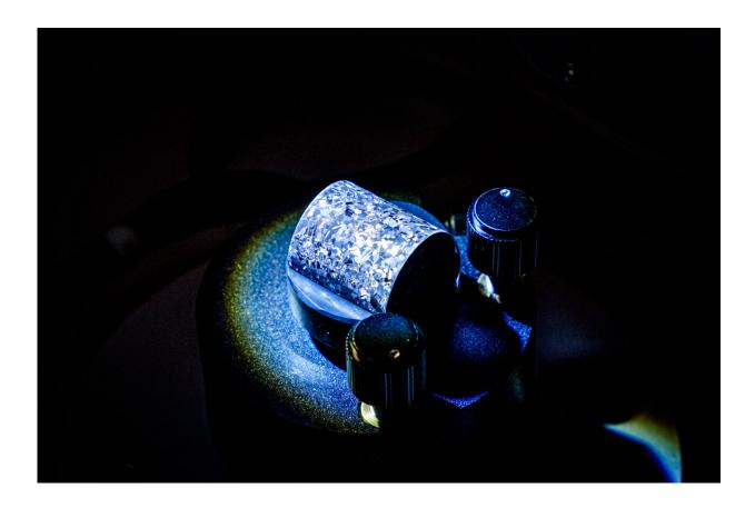
Analysing the unique crystals patterns on the surface of a 3D-printed metal may pave the way for the certification and quality assessment of parts made through additive manufacturing. Credit: Nanyang Technological University
