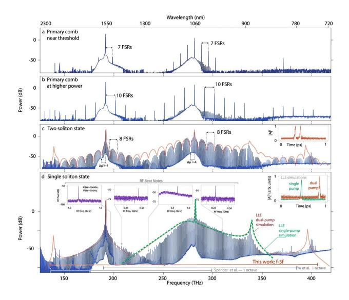
Spectral translation to create ultra-broadband microcombs. A microring resonator with RW = 1117 nm is pumped by a primary pump at 282 THz and synthesis pump at 192 THz. a Primary comb generation with low primary pump
