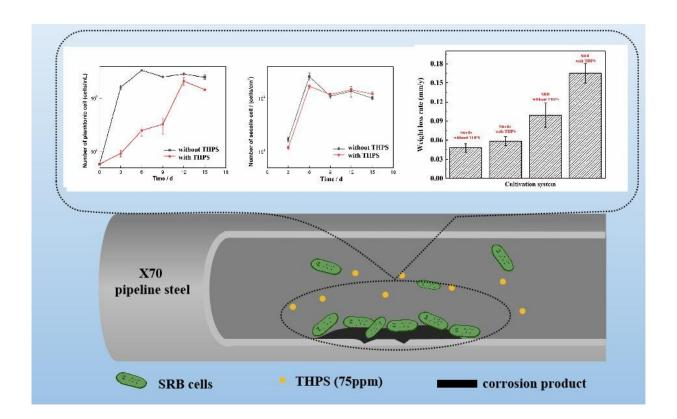
The illustration image of the MIC mechanism of pipeline steel under a tolerated THPS concentration (75 ppm) for D. hontreensis SY-21. Credit: IOCAS
