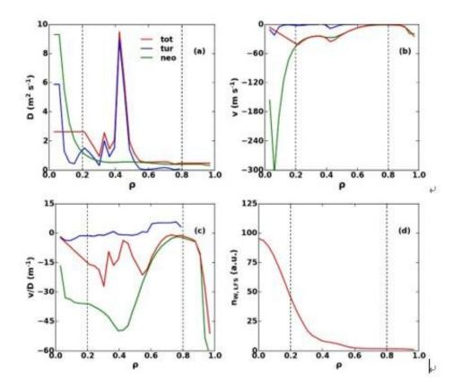
Radial profiles of (a) diffusion coefficient, (b) pinch velocity, (c) the ratio of pinch velocity to diffusion coefficient, (d) tungsten (W) density of 0 flux in the low field side in a hybrid discharge (shot #71326) on EAST. Credit: Shi Shengyu
