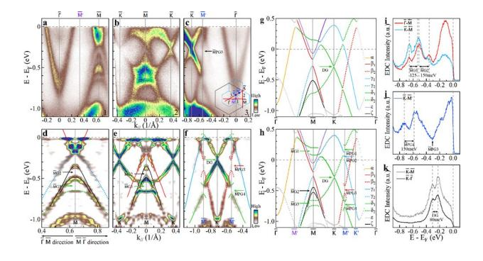
CDW-induced band splitting and gap opening in the measured band structures of  $KV_3Sb_5$  at 20 K and their comparison with band-structure calculations. Credit: Institute of Physics
