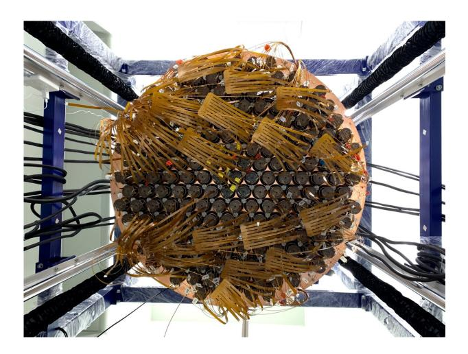
A plot of PMT arrays in the TPC detector of the PandaX-4T experiment. Credit: PandaX-4T Collaboration
