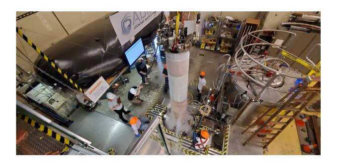
The ADMX apparatus right after extracting from the magnet bore. It was cooled by Liquid Nitrogen, so it makes cold mist. The left big black bag and right big reservoir are the parts of liquid Helium recycling system. Credit: ADMX Collaboration.
