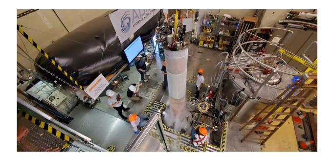
The ADMX apparatus right after extracting from the magnet bore. It was cooled by Liquid Nitrogen, so it makes cold mist. The left big black bag and right big reservoir are the parts of liquid Helium recycling system. Credit: ADMX Collaboration.
