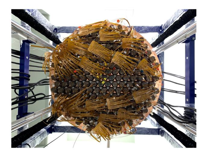
A plot of PMT arrays in the TPC detector of the PandaX-4T experiment. Credit: PandaX-4T Collaboration
