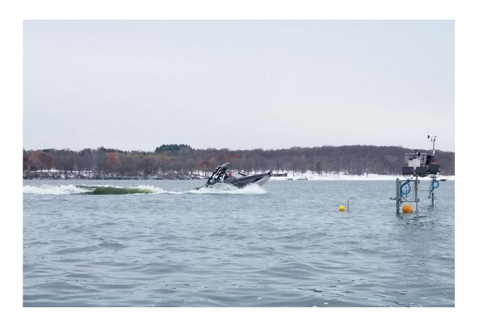
Researchers from the University of Minnesota St. Anthony Falls Laboratory carefully measured the maximum height, total energy, and maximum power of the waves from wakes produced by four recreational boats—two wakesurf boats and two more typical recreational boats. They also measured how the wake waves changed as they moved away from the boats and toward shore. Credit: Healthy Waters Initiative, University of Minnesota
