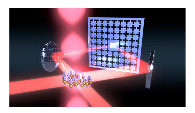
Light is used to couple a vibrating membrane to a cloud of atoms in order to form a control loop. The two different quantum systems — consisting of the membrane and the spins — therefore regulate one another's temperature with no need for external measurement. Credit: Department of Physics, University of Basel
