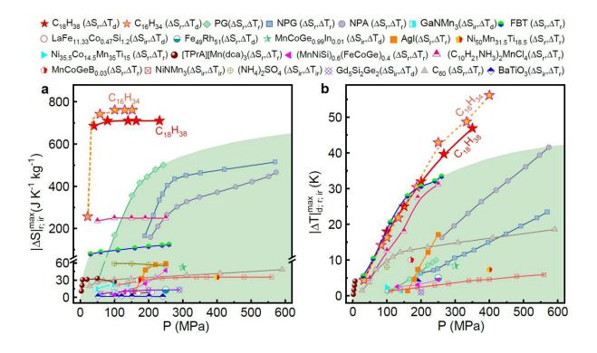
Comparision of BC performance between CnH2n+2 and the existing BC materials. The maximum adiabatic temperature change (a) and isothermal entropy change (b) as a function of pressure for C18H38 and C16H34, are shown along with the reported BC materials. Credit: Lin Jianchao
