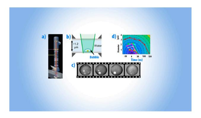
LLNL researchers combined a unique a) Dynamic Transmission Electron Microscope with b) a liquid cell to produce the first ever c) time resolved images of d) nanoscale bubble dynamics. Credit: Lawrence Livermore National Laboratory
