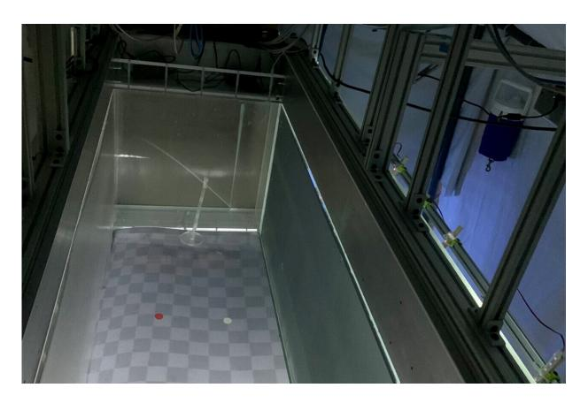
An image of the testing chamber and real-time, computer-based tracking system used to test the responses of flying mosquitoes to different visual objects, such as the colored dots at the base of the chamber. Credit: Kiley Riffell
