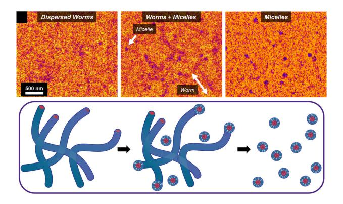
Processed LCTEM images showing worm-to-micelle transformations, induced by the flow of solvents. Credit: Northwestern University
