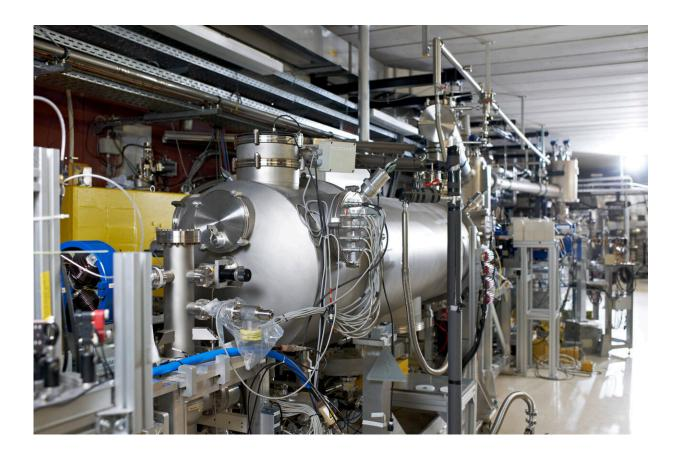
With this main module of ELBE, electrons can be accelerated to nearly the speed of light. In the SMART experiment, the particles generate "bremsstrahlung", which knocks out one neutron each from molybdenum atomic nuclei, leaving the radioisotope Mo-99. Credit: HZDR/Jürgen Jeibmann
