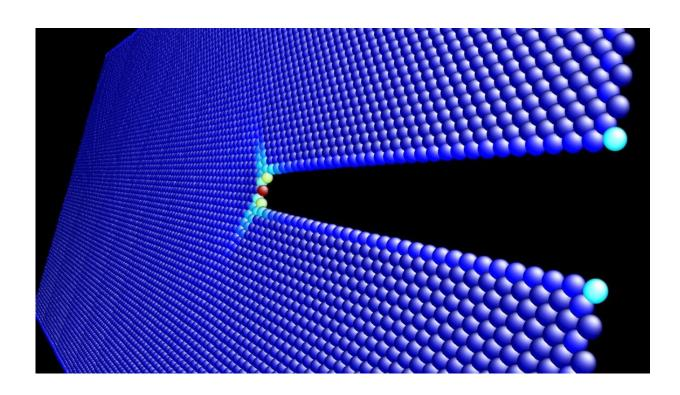
This rendering shows the modeled atomic configuration at the tip of a fatigue crack that is on the verge of emitting dislocation defects. Credit: Cornell University.
