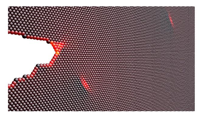
This rendering shows the modeled atomic configuration at the tip of a fatigue crack with two dislocation defects. Credit: Cornell University
