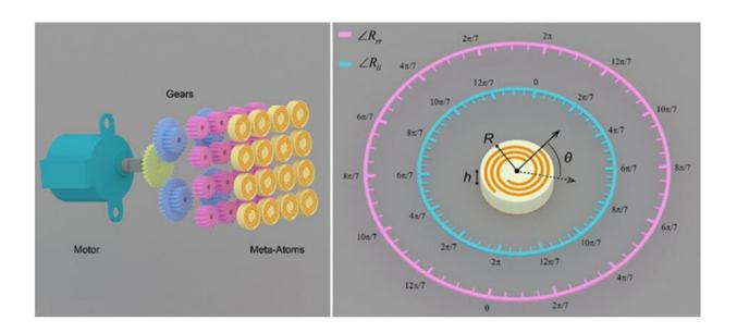
Schematic views of the RIS supercell and the meta-atom. Right: Geometric phase control in each supercell is achieved by transmitting the torque from a stepping motor to the meta-atoms through a set of gears. Left: Pink and sky-blue dials schematically depict the geometric phase control resolution and variation gradients for different circular polarizations. Credit: Xu et al
