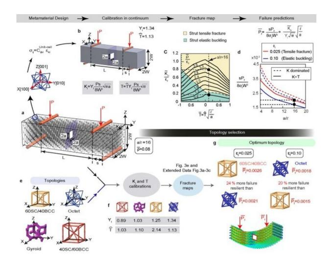
Design with metamaterials. (a) Octet-truss beam of aspect ratio L/W = 20 with the embedded crack (a/W = 0.2) subjected to four-point bending. (b) Geometry of the continuum anisotropic elastic beam used to determine the calibration factors YI and T^ for KI and T, respectively. (c) The cross-plotted fracture map from Fig. 3e. (d) Prediction of the normalized failure load Pf of the  $\rho^-$  = 0.08
