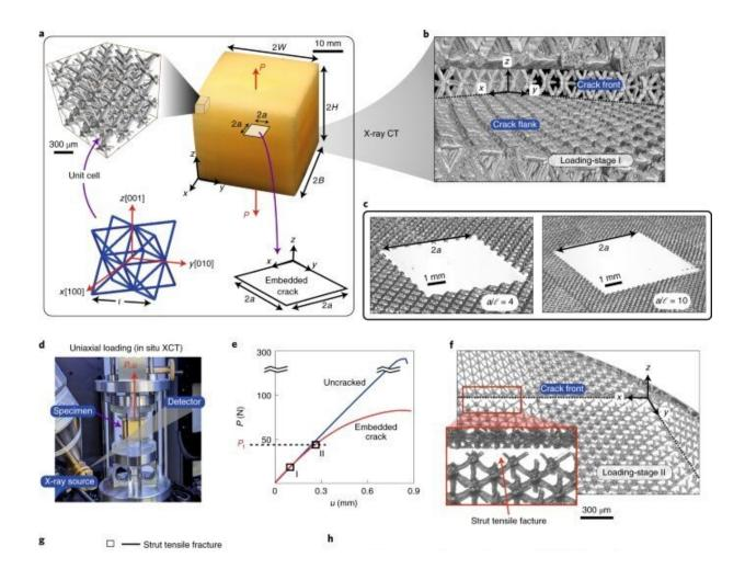
Failure under uniaxial tensile loading. (a) Optical image of the cubic octet-truss specimen with an embedded square crack of side 2a. Insets: XCT images of the octet-truss microstructure, unit cell and orientation and geometry of the embedded crack. b,c, XCT images of the crack front/flank at loading-stage I in e (b) and cracks of fixed size 2a but with varying cell sizes  $\ell$  as parameterized by
