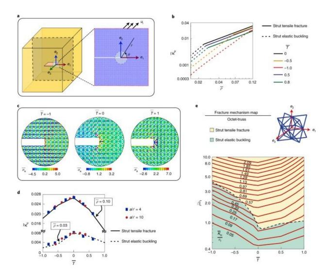
Fracture mechanism map. (a) Sketch illustrating the crack front coordinate system and a 2D slice used in the asymptotic analysis. (b) FE predictions
