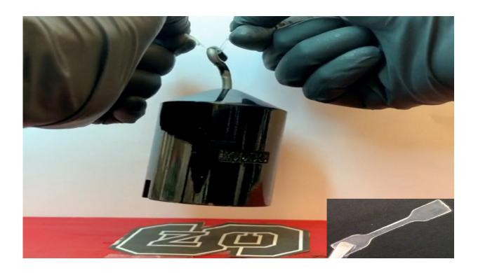
Researchers have created a material that is very stretchable and extremely tough. The material is of a type of ionogel, which is polymer network that contain salts that are liquid at room temperature. The new material has the stretchability of polyacrylic acid and is stronger than polyacrylamide. In terms of toughness, it's better than cartilage. A tab of the new material, shown in the lower left corner, is shown in this image supporting a weight. Credit: Meixiang Wang, NC State University
