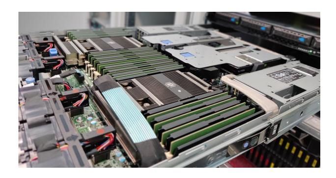
A candidate HLT node for Run 3, equipped with two AMD Milan 64-core CPUs and two NVIDIA Tesla T4 GPUs. (Image: CERN
