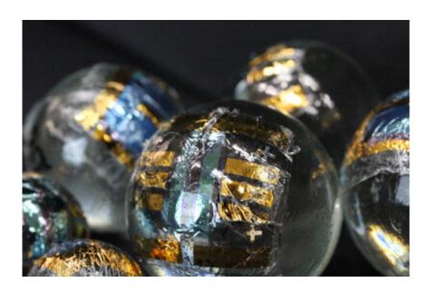
Figure 1: RIKEN researchers have used their heat-shrinking technology to attach organic photovoltaic films to spheres of different sizes. Credit: RIKEN Center for Emergent Matter Science
