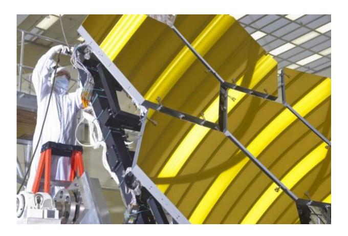
Webb's primary mirror undergoing cryogenic testing back in 2011. Credit: NASA
