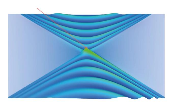
Hyperbolic shear polaritons are coupled light-matter waves that were discovered to exist at the surface of monoclinic crystals. Due to the low crystal symmetry, these waves are not mirror-symmetric. Credit: FHI / Wernerwerke
