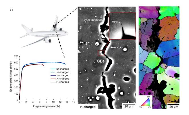
Tensile properties and metallographic fractography of an aluminum-based alloy with zinc, magnesium and copper after aging for 24 hours at 120°C. a) Engineering stress–strain curves of uncharged and hydrogen-charged samples. b and c) Electron imaging of an intergranular crack of the hydrogen-charged alloy subjected to tensile fracture. GB: grain boundary; GBPs: grain boundary precipitates. Credit: *Nature*
