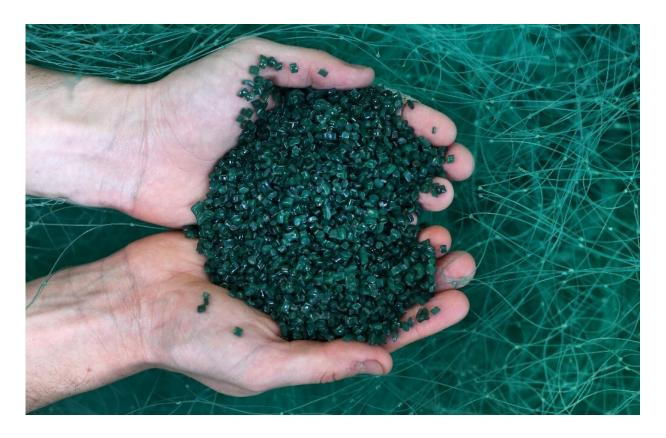
Net gains: French company Fil & Fab takes old fishing nets and turns them into nylon granules that are then incorporated in new products.
