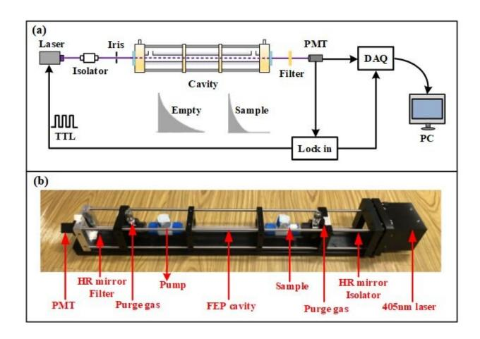
Schematic diagram of the experimental setup of the AM-CEAS instrument. Credit: Zhou Jiacheng
