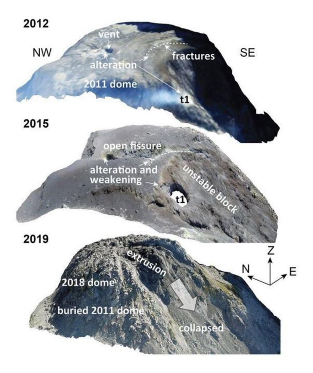
Nearly 10 yrs of drone surveys at Merapi volcano highlights the importance of hydrothermal weakening and structures hidden beneath younger lavas. A fracture system that formed in 2012 was subsequently buried under new lava in 2018. Only a year later, the new lava dome that formed in 2018 showed signs of
