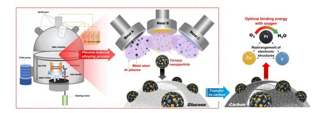
Illustration of the step-by-step synthesis process for the preparation of ternary nanoparticle catalysts and electron structure rearrangement by electron transfer between metal atoms. Credit: Korea Institute of Science and Technology (KIST)
