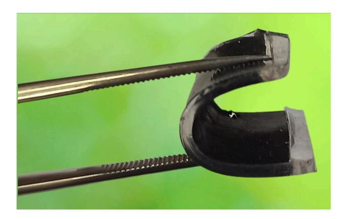
Tongs bending a flexible supercapacitor into a U shape. Credit: University of Surrey
