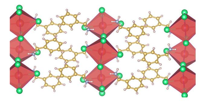
A typical structure of two-dimensional perovskites. Credit: Los Alamos National Laboratory
