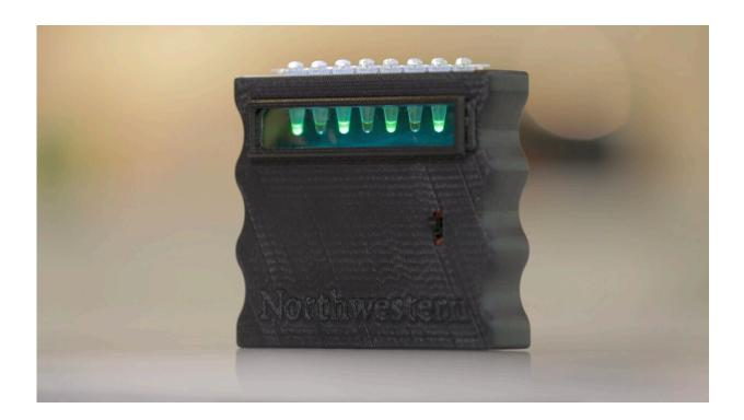
Test tubes holding water samples glow green inside an illuminator, indicating contamination. Credit: Northwestern University
