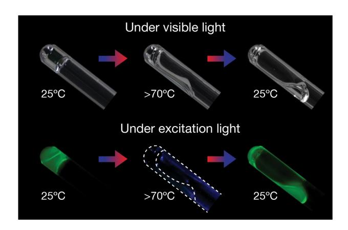
(Top) The star-polymer-DNA-gel (left) liquifies when its temperature is increased to more than 70°C (center), and returns to a gel when the temperature drops back to 25°C (right). (Bottom) Under UV light, the star-polymer-DNA-gel fluoresces green (left, right), but does not fluoresce when liquified (Photo: Xiang Li). Credit: Xiang Li
