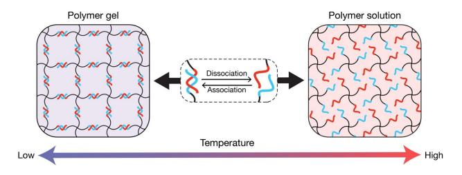
The star-polymer-DNA gel consists of complementary DNA strands (red and blue) linked to a molecule called polyethylene glycol (PEG, black). At lower temperatures, the DNA strands form complementary bonds leading to a gel; as the temperatures increase, the complementary bonds break and the gel liquifies. Credit: Masashi Ohira et al, *Advanced Materials*, January 16, 2022
