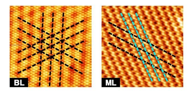
Figure shows the charge density waves imaged using scanning tunnelling microscopy for (left) bilayer (BL)-VSe<sub>2</sub> and (right) monolayer (ML)-VSe<sub>2</sub>. Dashed colour-coded lines represent the wavefronts for the 4a (black) and 2.8a (cyan) charge density waves (CDWs) respectively. Credit: *ACS Nano*
