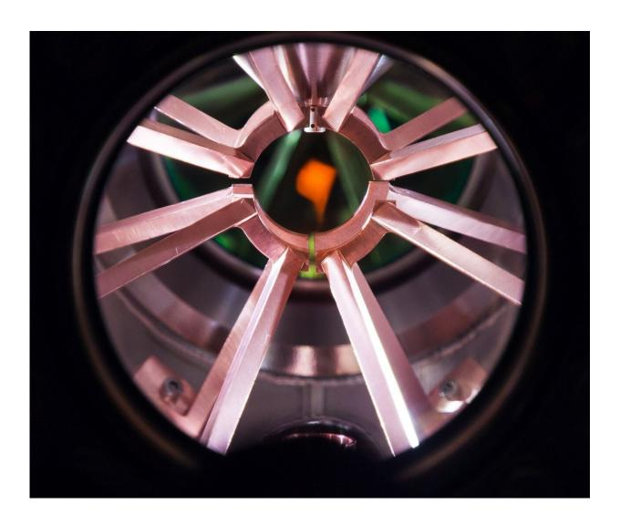
Ultracold atomic cloud of rubidium atoms used in this experiment: You can see the fluorescence that occurs during laser cooling. Credit: AG Ott/TUK
