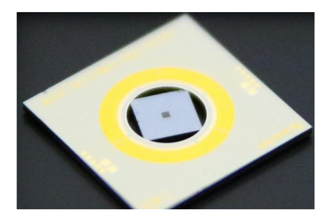
The researchers suspended a metasurface on square silicon chip in a thin-film PZT MEMS-actuated ring (yellow). Credit: Christopher Dirdal, SINTEF Smart Sensors and Microsystems
