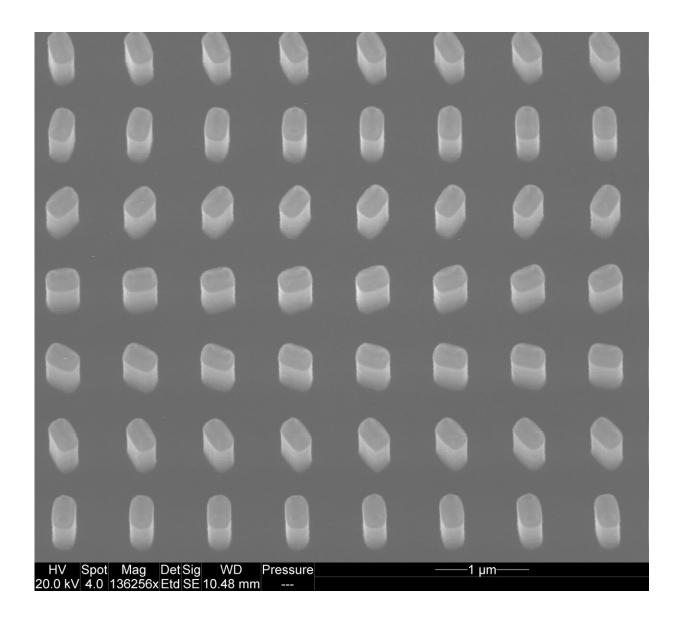
This electron microscopy image shows the nanostructure of the metasurface located at the center of the suspended silicon chip. The spacing from pillar to pillar is 835nm, around 50 times thinner than a strand of hair. Credit: Christopher Dirdal, SINTEF Smart Sensors and Microsystems
