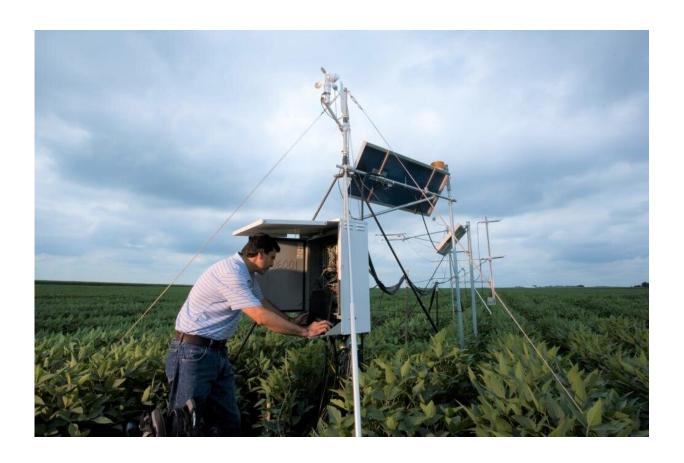
Researcher Suat Irmak programming the datalogger in one of his surface water vapor and energy flux towers to measure crop water use, all incoming and outgoing radiation fluxes, and all other climate variables such as air temperature, relative humidity, vapor pressure deficit, net radiation, precipitation, soil moisture, soil temperature on an hourly basis. The same flux tower was used in this corn vs. climate change study. Credit: Suat Irmak research group. All rights
