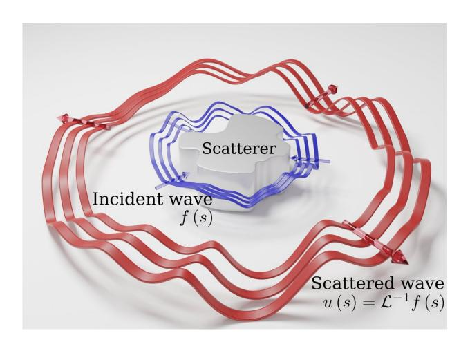
Scattered waves from a nanoscale object encode the solution of a complex mathematical problem when interrogated by tailored input signals. Credit: Heedong Goh
