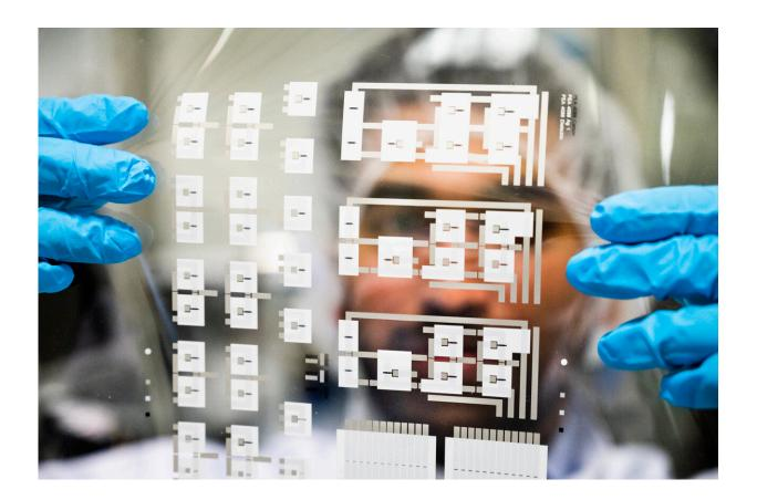
The researchers have shown that thousands of organic chemical transistors can be printed in a small area on thin plastic foil. Credit: Thor Balkhed
