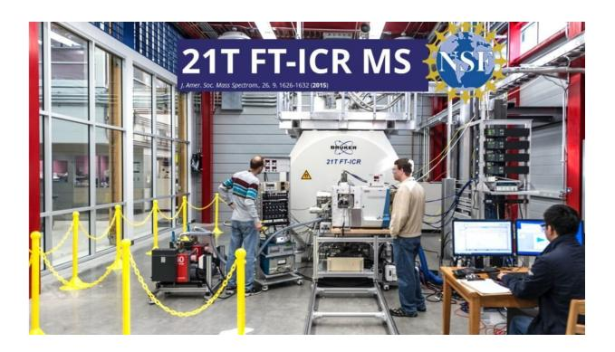
The 21 tesla Fourier-transform ion cyclotron resonance mass spectrometer (21T FT-ICR MS) at the NSF-funded National High Magnetic Field Lab is the most powerful, highest resolving machine of its kind. It uses electric and magnetic fields to distinguish individual molecules and can differentiate between chemical compounds more accurately than any other instrument. Credit: Colorado State University
