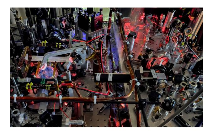
Experimental setup with laser-cooled rubidium atoms, which process the quantum data in visible light (left). Experimental setup of the laser beam, which programs quantum operations carried out in light trapped inside the atoms (right). Credit: University of Warsaw
