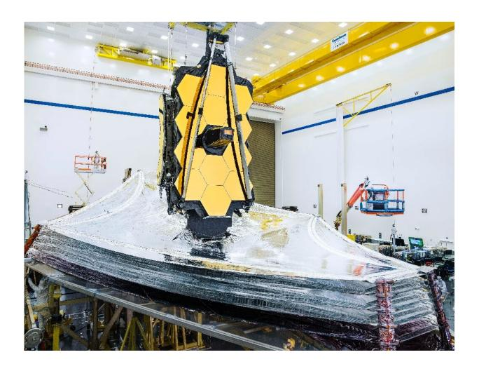
The tennis court size, kite-shaped apparatus acts like a parasol, ensuring the observatory is kept in the shade so that it is able to detect faint infrared signals from the far reaches of the Universe.
