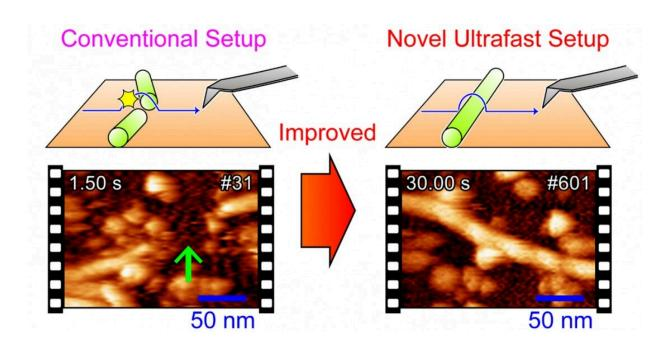
Comparison of AFM images taken by conventional and ultrafast amplitude detector. A novel ultrafast amplitude detector developed in the present study allows us to perform low-invasive high-speed AFM imaging for biological samples. Now, actin filaments, one of the cytoskeletal protein filaments in eukaryotic cells, can be successfully imaged at video rate without breaking them. Credit: Kanazawa University
