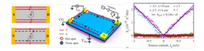
Left panel: Downstream (red lines) and upstream (dashed black lines). Middle panel: Schematic for noise measurement for "upstream" mode detection. Right panel: Noise is detected for fractional quantum Hall states with "upstream" modes whereas it remains zero for only downstream modes. Credit: Authors
