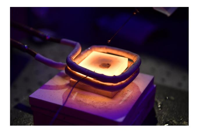
The STA successfully inhibits the occurrence of the Leidenfrost effect even up to 1,150 °C and achieves efficient liquid cooling. Credit: City University of Hong Kong
