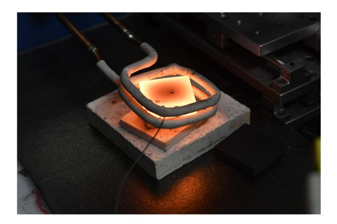
In the Leidenfrost effect, an insulating vapor layer is produced and heat transfer is dramatically reduced. Credit: City University of Hong Kong
