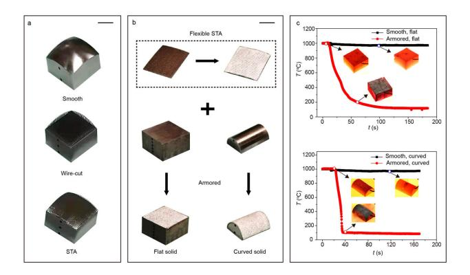
(a) A smooth spheroidal piece of steel can be covered by thick pillars after wire cutting. Inserting a membrane in the pillars provides a curved STA. (b) STA can also be made on thin films of steel, which makes it flexible. The films can be welded onto flat or cylindrical solids. (c) The armours are tested to be able to provide rapid and efficient cooling, as evidenced by the drop in temperature (red data). Credit: Jiang, M. et al.
