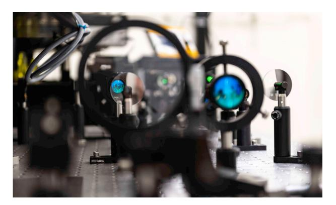
Close-up of the laser system in Andrea Pickel's lab, located in Hopeman Hall. The researchers use green laser pulses to excite the nitrogen vacancy centers in the nanodiamonds in order to send the electrons into a higher energy state. Credit: University of Rochester photo / J. Adam Fenster
