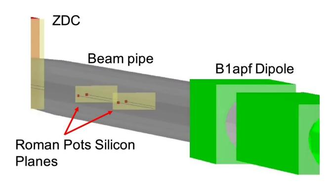
Zoomed-in image of a 3BBU-MF  $e+{}^{3}$ He with both protons tagged in the Roman Pot silicon detector planes. The beam pipe was made semi-transparent in order to see the event. The off-momentum detectors are omitted from the figure to make the event easier to view. Credit: DOI: 10.1016/j.physletb.2021.136726
