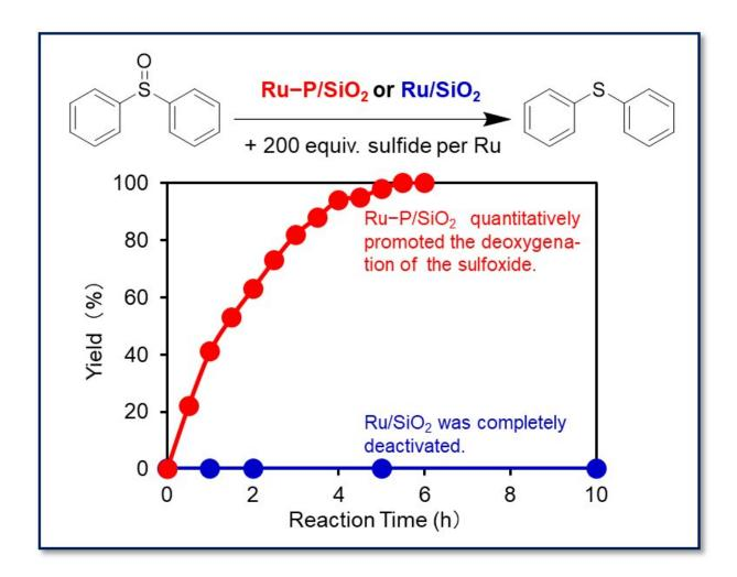
Fig. 2. Catalytic performances of Ru–P/SiO<sub>2</sub> and Ru/SiO<sub>2</sub> for the sulfoxide deoxygenation in the presence of sulfide. Credit: Osaka University
