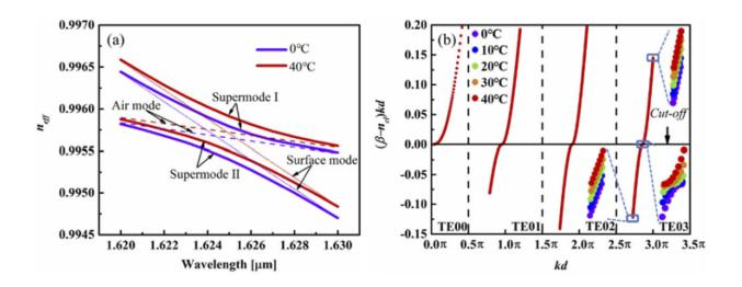
Fig. 1. (a) Simulated supermode dispersions at the avoided crossing of typical PBG-HCF at 0°C and 40°C. The dashed lines show dispersions of independent air (dash) and surface (dot) modes without coupling. (b) The normalized effective refractive indices of TE0m modes in an air-cladding silica glass slab waveguide at different temperatures when thermo-optic effect and thermal expansion are considered. Credit: DOI: 10.1364/OE.443075
