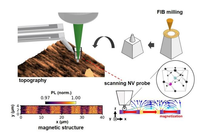
Imaging of domain structure in a magnetic tape with a scanning NV probe. Scanning diamond NV center probe fabricated by FIB milling demonstrates imaging of magnetic domain structure of magnetic tape. Credit: Toshu An from JAIST.
