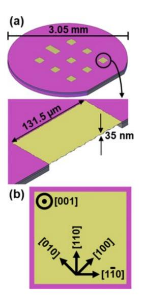
Schematic drawing showing (a) grid and membrane dimensions and (b) crystallographic directions. 3.05 mm corresponds to standard transmission electron microscope (TEM) grid size, while window dimensions and crystal directions are a result of the anisotropic wet etching of silicon-on-insulator (SOI)
